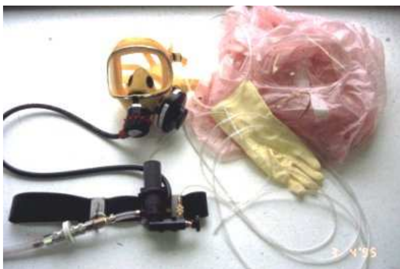
Figure 2. Combined breathing and cooling air supply to operators in ventilated clothing
