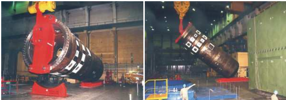
Figures 6. & 7. Tilting device for the reactor components
