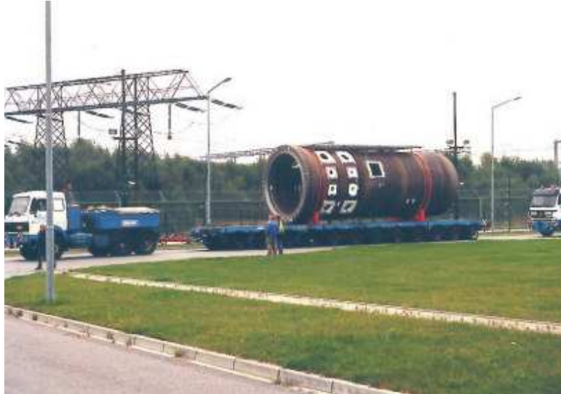
Figure 5. Transport of the RPV of unit 8 to unit 5
