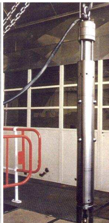
Figure 8. Combined standpipe cutter/grab
