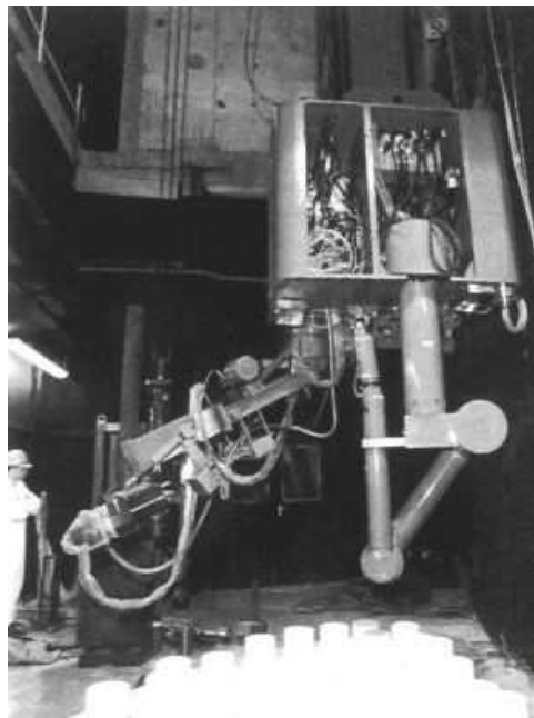
Figure 13. Remote Dismantling Machine Test Facility working on polystyrène mock-up
